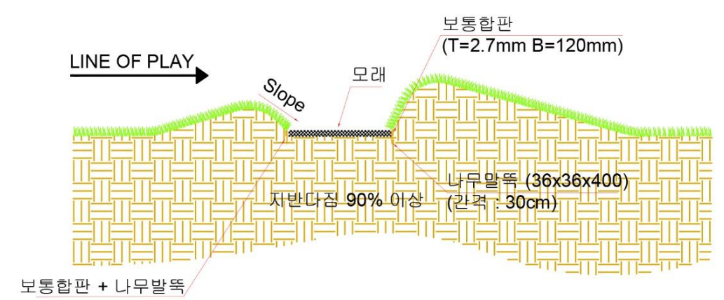
3 G bunker cross-section scale = 1/100
